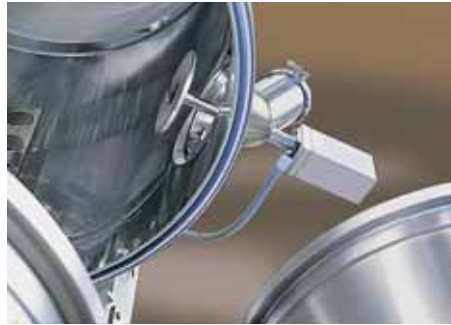
Charge port flush with the wall
