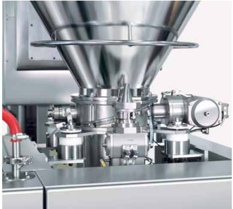
Charging with the SKS valve system
