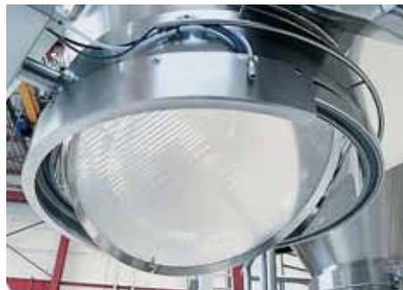
Wedge-wire turning bottom for vertical discharge
